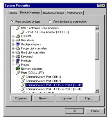
Click the **B&B Electronics Serial Adapters** device to view the adapter. If you want other details, Select **Properties**.
